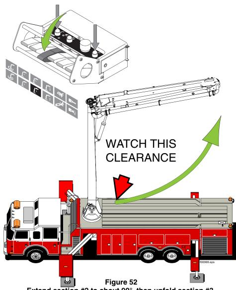
Extend section #2 to about 90°, then unfold section #3.
